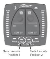
The ATP Helm Control allows for the user to set two different favorite positions. These positions are a combination of pitch and roll attitudes that the user feels are comfortable or useful running attitudes for the boat.
