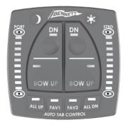
These LEDs represent the range of motion that the trim tabs may move through. The four yellow LEDs will be illuminated continuously during normal operation. If one of the upper yellow LEDs is flashing, this is an indication to the user that the system is not receiving a signal from one of the actuator sensors (see page 20).
