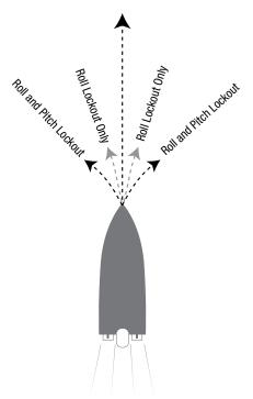
boat is in a turn and modify the way that it tries to adjust. If the turn is fairly gradual (less than 1 degree per second) the ATP control will still make adjustments to the boat to compensate for pitch changes. These pitch changes are uniform on both
