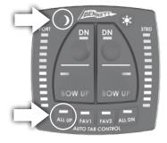
This will set the resting position of the boat and allow the system to retract the trim tabs any time that the system detects the boat is at rest.
