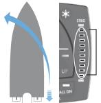
When the Stbd. tab is lowered (deployed), the Stbd. red LEDs on the ATP display will illuminate. As a result, the port (left) bow will lower.
