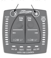
The Sun and moon buttons are used to increase and decrease the brightness of the LEDs on the display.
