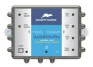
The ATP Control Unit is the sensor and processor for the ATP system which activates the electric actuators that adjust the trim tabs. The unit contains an accelerometer, gyroscope, and an electronic compass that sense the position and movements of the boat and therefore should not be mounted within 24" of any magnetic items such as electric motors or speakers. However, the ATP Control Unit can be conveniently mounted anywhere in the boat, and in any orientation.
